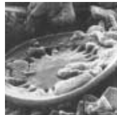
SeitzSchenk Depth Filter Sheets—microscopic morphology of diatomaceous earth
