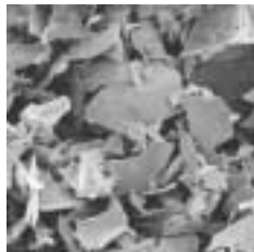
SeitzSchenk Depth Filter Sheets—microscopic morphology of perlites
